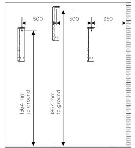
To comply with AS2890.3 (2015) minimum 500mm spacing between rack centres and 350mm to edge of walls or other obstructions, with racks at alternating heights.
