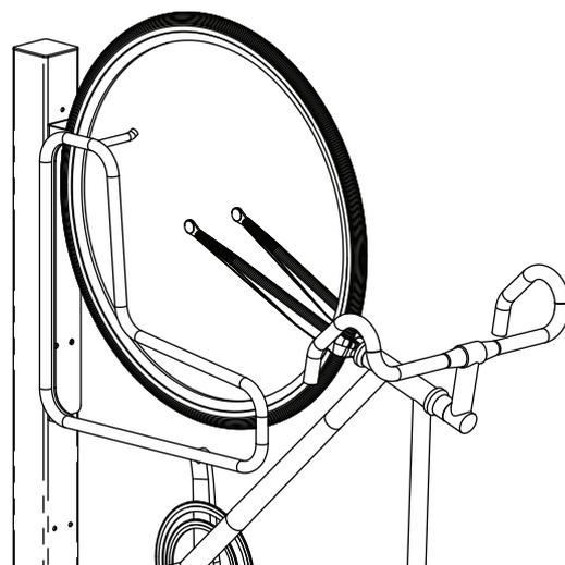
**3** Ensure the rear wheel is resting within the wheel holder. Secure bike to rack using personal locking device. Cora recommends locking the bike frame and at least one wheel to the rack.
